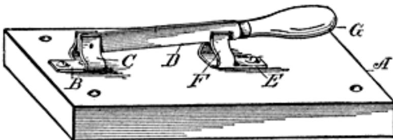
*Fig. 43.* Two-Pole Switch
