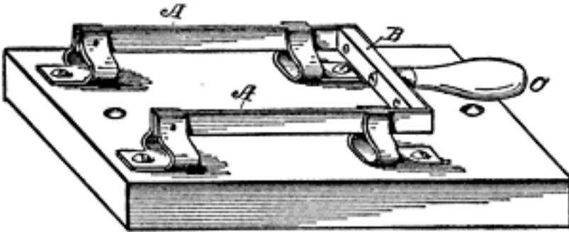
Fig. 44. Double-Pole Switch
