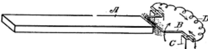
Fig. 102. Cutting a Magnetic Field
